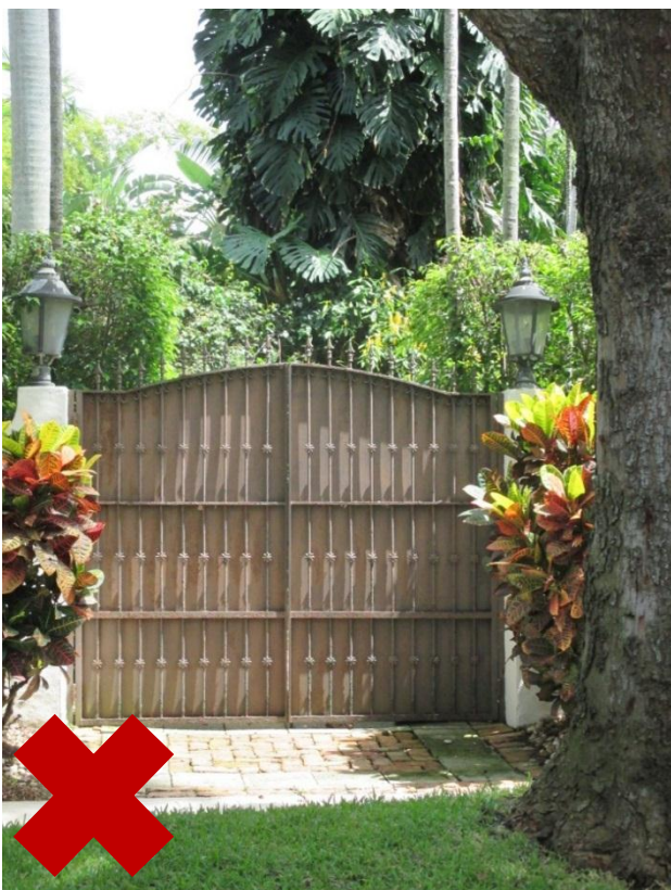
FIGURE 4.4 Gates and fencing in the first layer shall have at least 60% visibility
